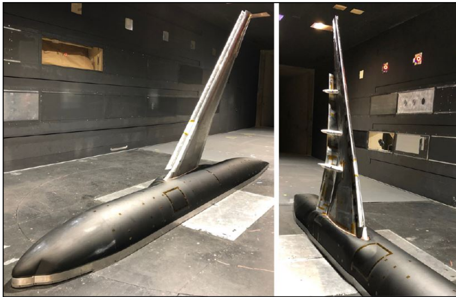
Figure 6-8. Semi-span CRM-HL model installed in the NASA LaRC 14x22 Foot Wind Tunnel
