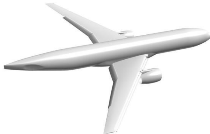
Figure 6-7. High Lift Common Research Model geometry
